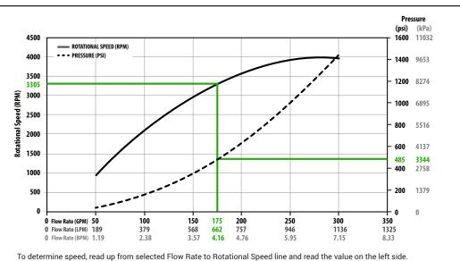
To determine pressure, read up from selected Flow Rate to Pressure line and read the value on the right side.
