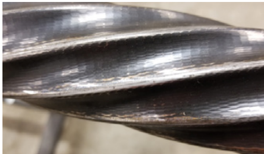
Figure 2 - Closeup of rotor contact patch
