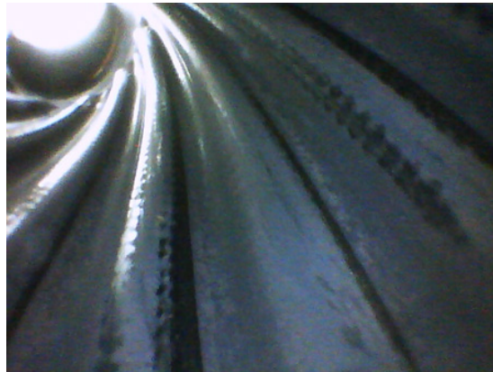
Figure 4 - Post-run borescope of stator
