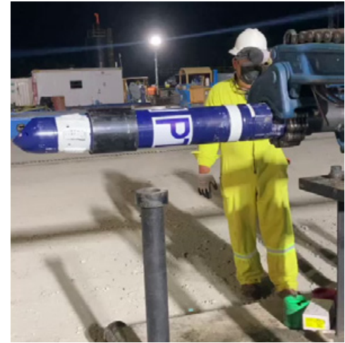
Preparing the third HSRT prior to starting the casing run.
