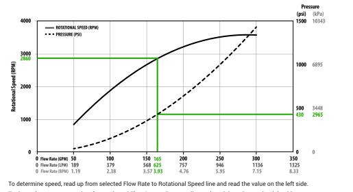
To determine pressure, read up from selected Flow Rate to Pressure line and read the value on the right side.
